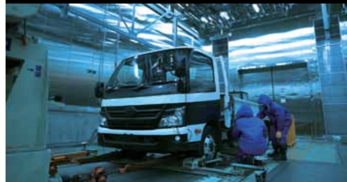
Durability tests were conducted in an environmental test chamber under temperatures ranging from +50 to -40°C.
