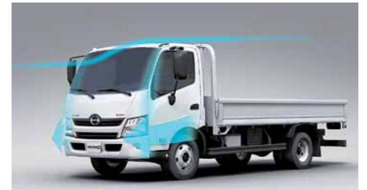
Fig. 1: The larger corner radius and cabin shape that is tapered towards the front contribute to improved aerodynamic performance.
