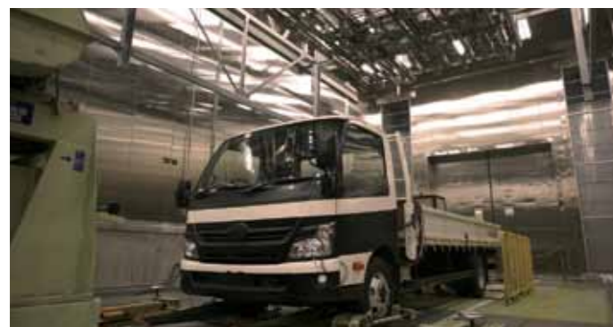
Durability tests were conducted in an environmental test chamber under temperatures ranging from +50 to -40°C.
